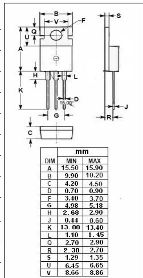
**isc N-Channel MOSFET Transistor      IRFB23N15D, IIRFB23N15D****ELECTRICAL CHARACTERISTICS****T<sub>c</sub>=25°C unless otherwise specified**
