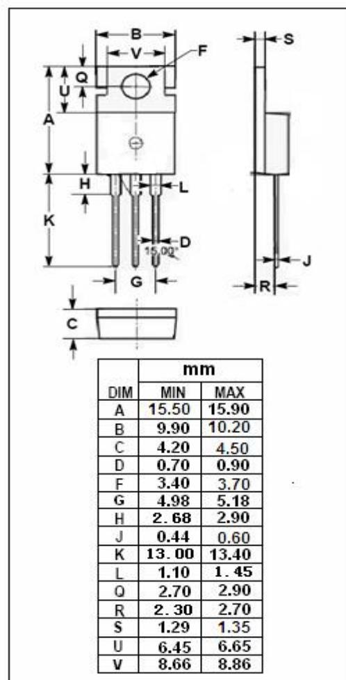
**isc N-Channel MOSFET Transistor****IRFB3206,IIRFB3206****ELECTRICAL CHARACTERISTICS****T<sub>c</sub>=25°C unless otherwise specified**
