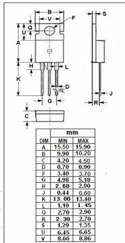
**isc N-Channel MOSFET Transistor****IRFB3207, IIRFB3207****ELECTRICAL CHARACTERISTICS****T<sub>C</sub>=25°C unless otherwise specified**
