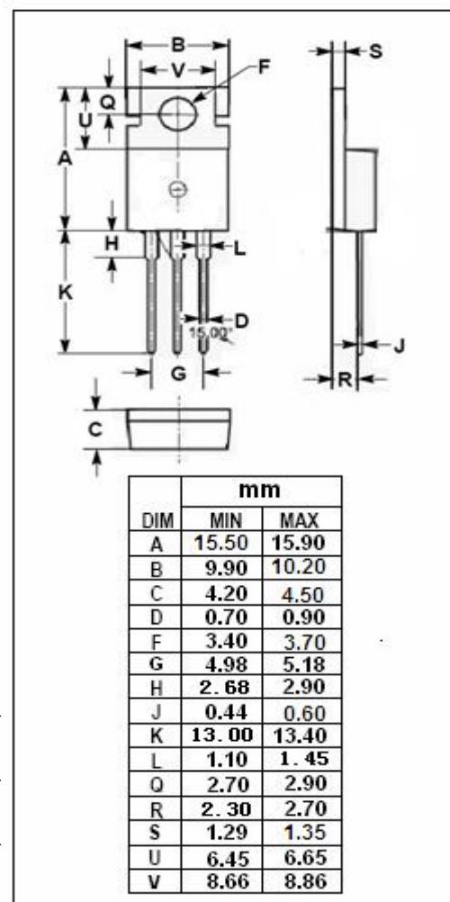
**isc N-Channel MOSFET Transistor****IRFB4115, IIRFB4115****ELECTRICAL CHARACTERISTICS****T<sub>c</sub>=25°C unless otherwise specified**
