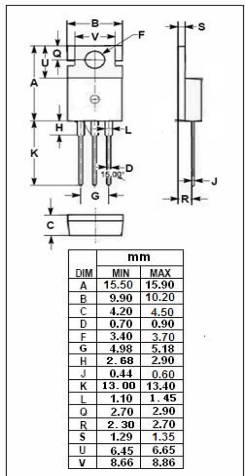
**isc N-Channel MOSFET Transistor****IRFB7740, IIRFB7740****ELECTRICAL CHARACTERISTICS****T<sub>c</sub>=25°C unless otherwise specified**
