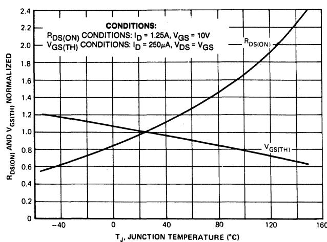
TYPICAL NORMALIZED  $R_{DS(ON)}$  AND  $V_{GS(TH)}$  VS. TEMP.
