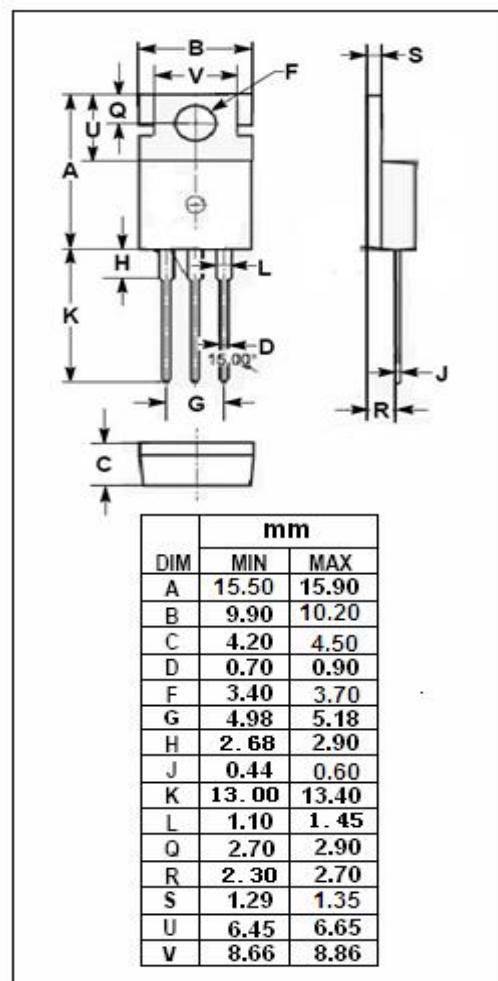
**isc N-Channel MOSFET Transistor****IRFL3713,IIRFL3713****ELECTRICAL CHARACTERISTICS****T<sub>c</sub>=25°C unless otherwise specified**
