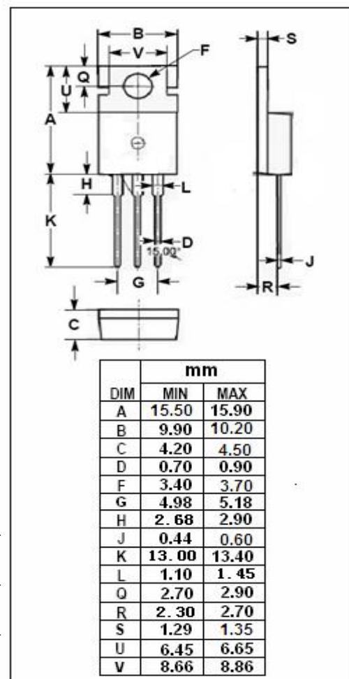
**isc N-Channel MOSFET Transistor****IRFZ48V, IIRFZ48V****ELECTRICAL CHARACTERISTICS****T<sub>C</sub>=25°C unless otherwise specified**
