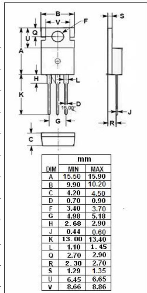
**isc N-Channel MOSFET Transistor****IRL3103, IIRL3103****ELECTRICAL CHARACTERISTICS****T<sub>c</sub>=25°C unless otherwise specified**
