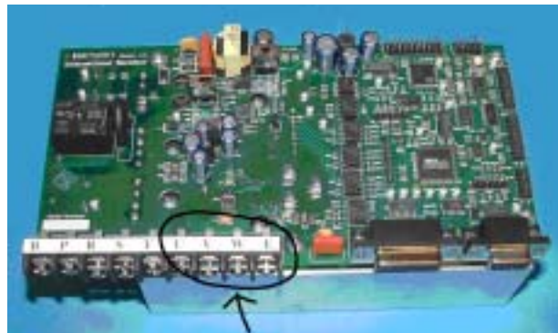
Figure 4. Motor Wiring Connection
