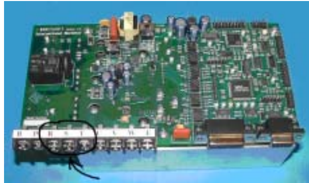
Figure 3. Power Terminal Block, J1
