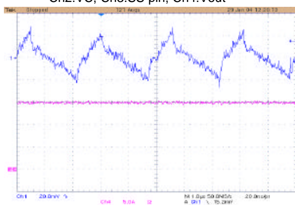
Figure 17 - Output Voltage Ripple @ 15A Ch1:Output, Ch4:lout (5A/Div)
