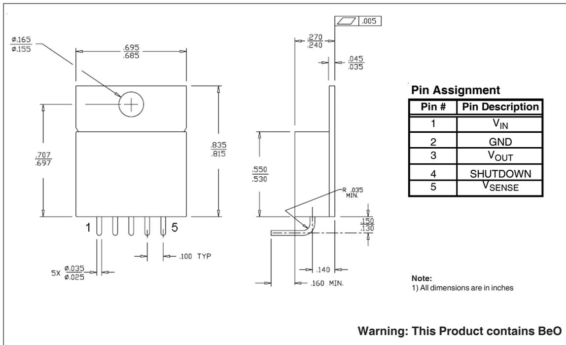
**Fig 9. Case Outline and Dimensions - MO-078AA (Lead Trimmed)**
