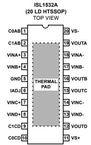
\*THERMAL PAD DOWN-BONDED TO GND
