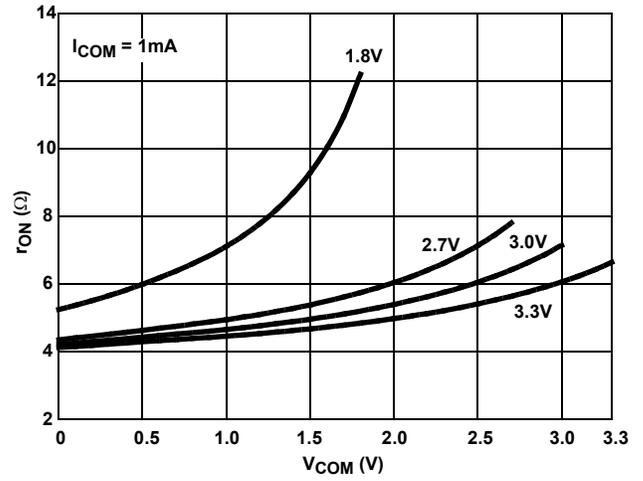
FIGURE 8. ON-RESISTANCE vs SUPPLY VOLTAGE vs SWITCH VOLTAGE
