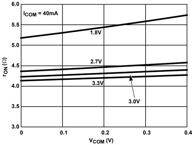
FIGURE 7. ON-RESISTANCE vs SUPPLY VOLTAGE vs SWITCH VOLTAGE
