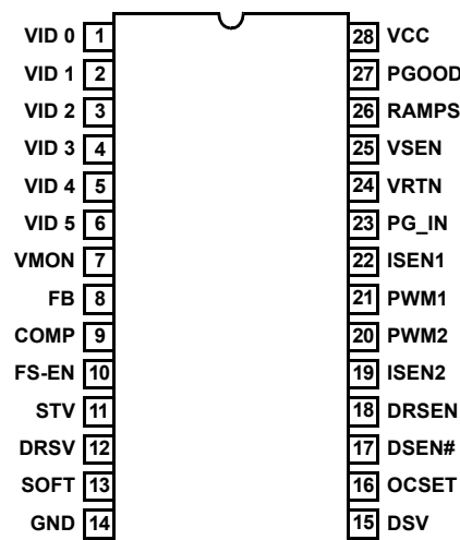
ISL6216 (28 LEAD SSOP) TOP VIEW
