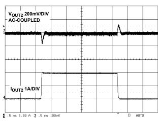
FIGURE 8. LOAD TRANSIENT RESPONSE V<sub>OUT2</sub> (3.3V)
