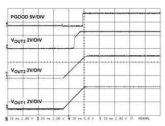
FIGURE 4. SOFT-START WAVEFORMS WITH PGOOD
