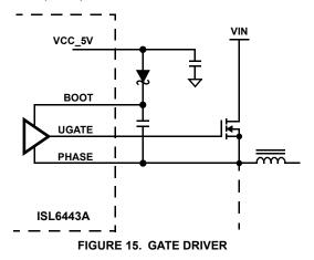
At start-up, the low-side MOSFET turns on and forces PHASE to ground in order to charge the BOOT capacitor to 5V. After the low-side MOSFET turns off, the high-side MOSFET is turned on by closing an internal switch between BOOT and UGATE. This provides the necessary gate-to-source voltage to turn on the upper MOSFET, an action that boosts the 5V gate drive signal above  $V_{\text{IN}}$ . The current required to drive the upper MOSFET is drawn from the internal 5V regulator.
