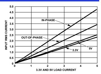
FIGURE 20. INPUT RMS CURRENT vs LOAD
