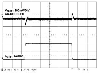
FIGURE 7. LOAD TRANSIENT RESPONSE  $V_{OUT1}$  (3.3V)
