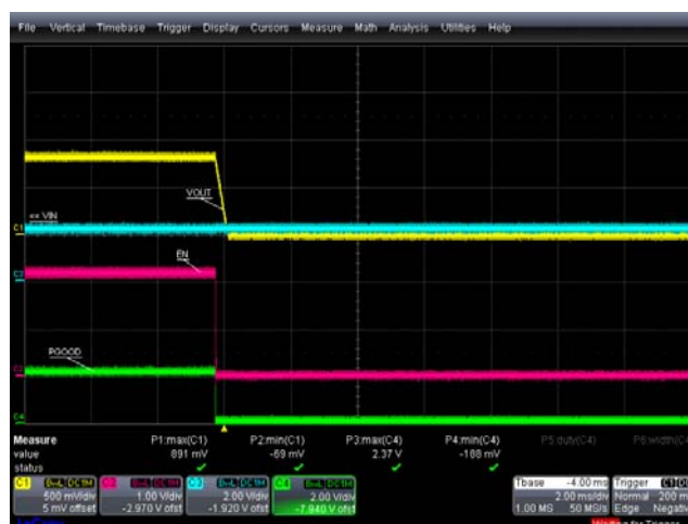
FIGURE 26. POWER-ON AND POWER-OFF, EN = 1 TO 0, +25°C, VIN = 2.2V, VOUT = 0.8V, IOUT = 0.5A, PGGOOD TURN-OFF
