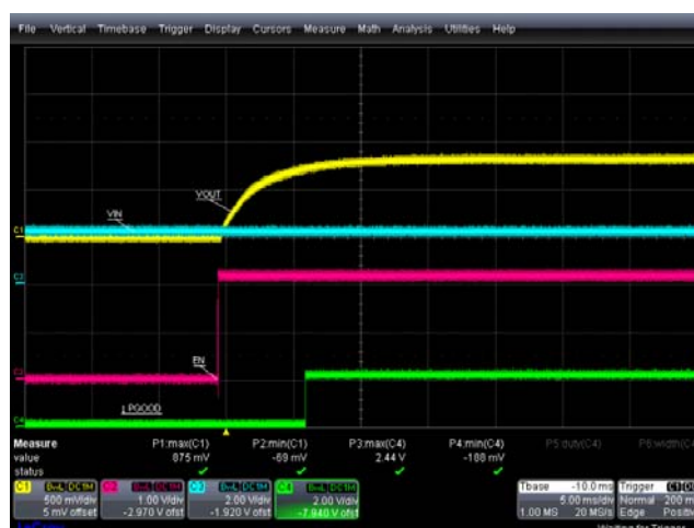
FIGURE 24. POWER-ON AND POWER-OFF, EN = 0 TO 1, +25°C, VIN = 2.2V, VOUT = 0.8V, IOUT = 0.5A, PGGOOD TURN-ON
