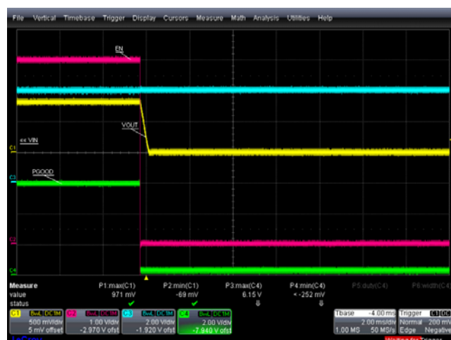
FIGURE 25. POWER-ON AND POWER-OFF, EN = 1 TO 0, +25°C, VIN = 6V, VOUT = 0.8V, IOUT = 0.5A, PGGOOD TURN-OFF
