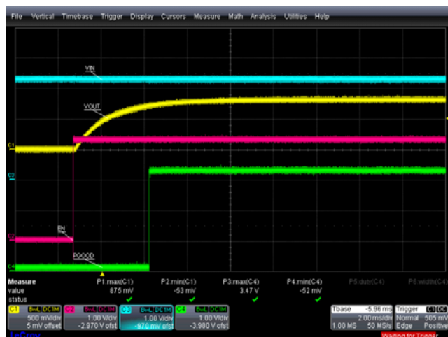
FIGURE 23. POWER-ON AND POWER-OFF, EN = 0 TO 1, +25°C, VIN = 6V, VOUT = 0.8V, IOUT = 0.5A, PGGOOD TURN-ON
