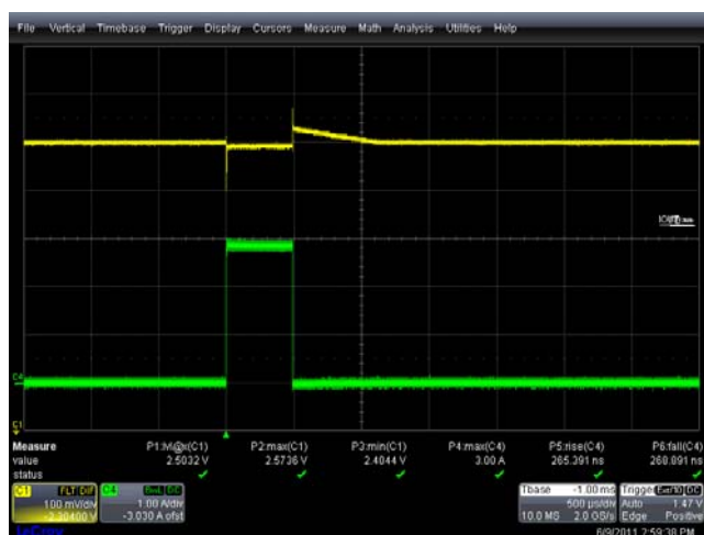
FIGURE 21. TRANSIENT LOAD RESPONSE, V_{IN} = 3.3V , V_{OUT} = 2.5V , C_{OUT} = 47\mu F , 35m\Omega
