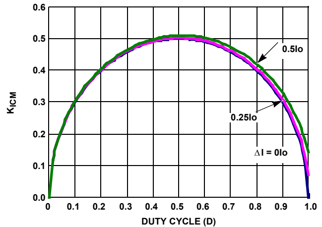
FIGURE 11. INPUT-CAPACITOR CURRENT MULTIPLIER FOR SINGLE-PHASE BUCK CONVERTER
