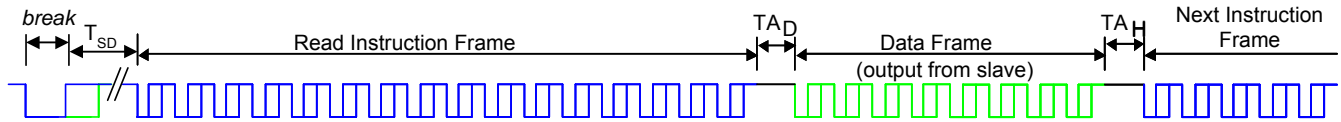
FIGURE 10. XSD BUS TRANSACTION PROTOCOL. THE 'BREAK' SIGNAL IS OPTIONAL IF THE DEVICE IS AWAKE
