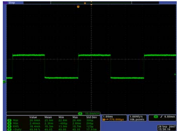
FIGURE 16. I LED AT 50% PWM DIMMING
