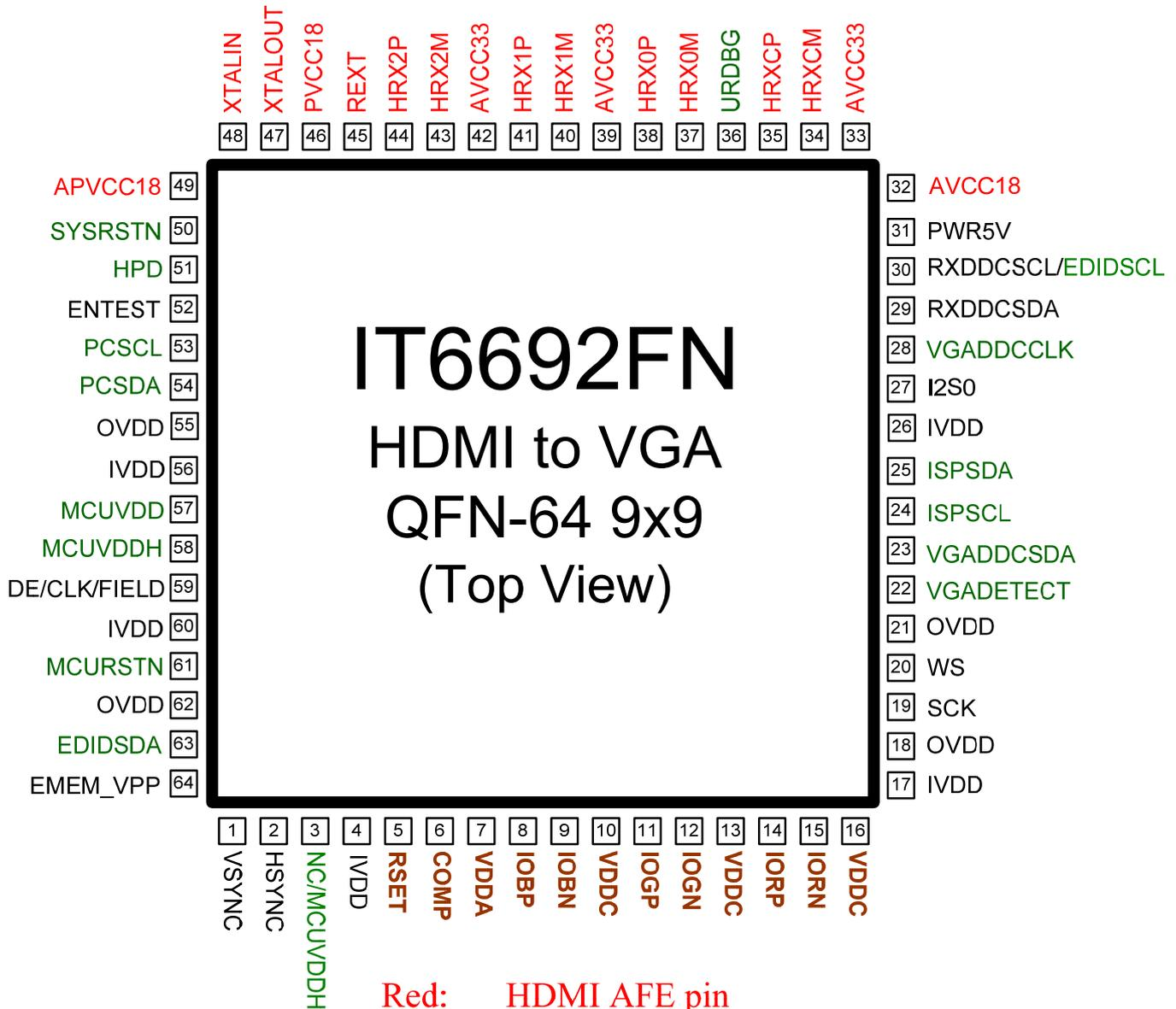
Figure 1. IT6692FN pin diagram
