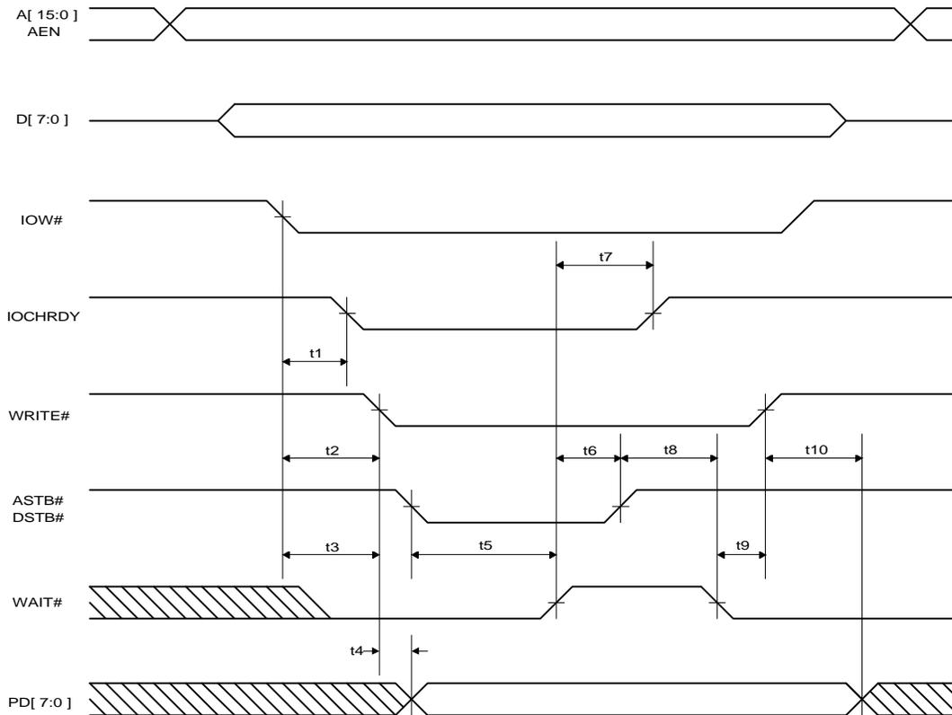
**Table 9-16. EPP Address or DATA WRITE Cycle**
