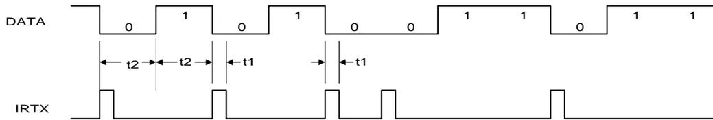
PULSE WIDTH  $t_1 = 3/16$  OF BIT TIME  $t_2$
