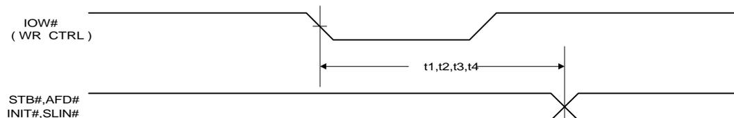
**Table 9-14. Control Signal Delay Time of Parallel Port Timing**
