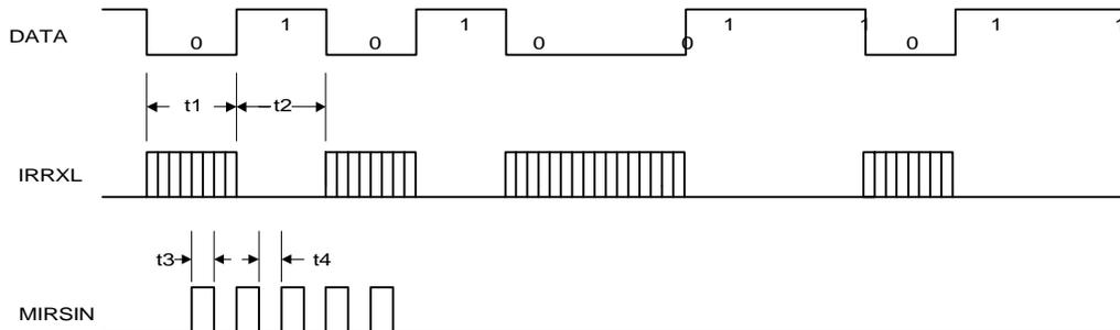
**Table 9-12. ASKIR Receive Timing of Serial Port Timing**
