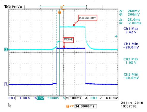
Below timing diagram of IBX EDS demonstrate power sequence from S3 to S0, the relation between PCH core 1.05V and PWROK are described when PCH core 1.05V is ready minima 10ms after PWROK active.
