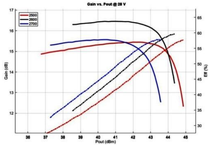
Figure 2. Power gain and drain efficiency as function of Pulse output power (2500-2700MHz)
