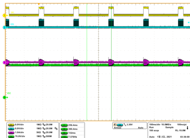
Light Load Burst with DC Input
