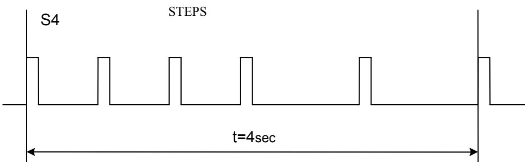
$$\text{Rate} = (5 \text{ steps}/4 \text{ seconds}) * 60 \text{ seconds} = 75 \text{ steps per minute}, \text{ C RATE}=8;$$
