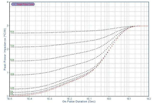
Transient Thermal Response Curve For JCS4N60FB(TO-220MF)
