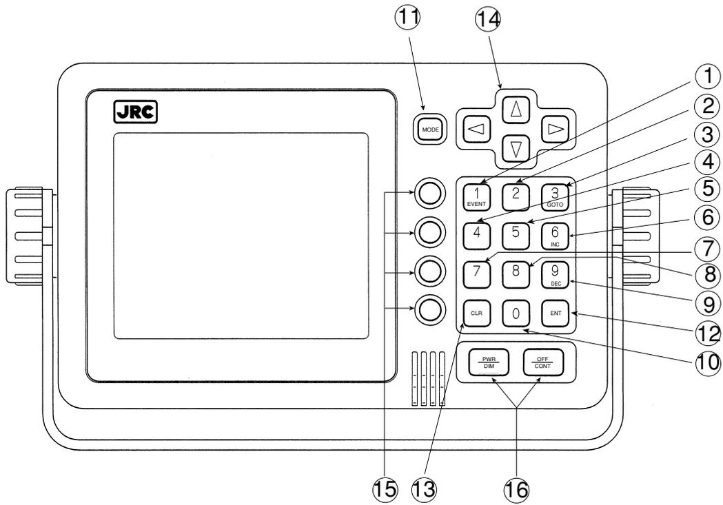
Fig. 2-1 Operation Panel of the Navigator
