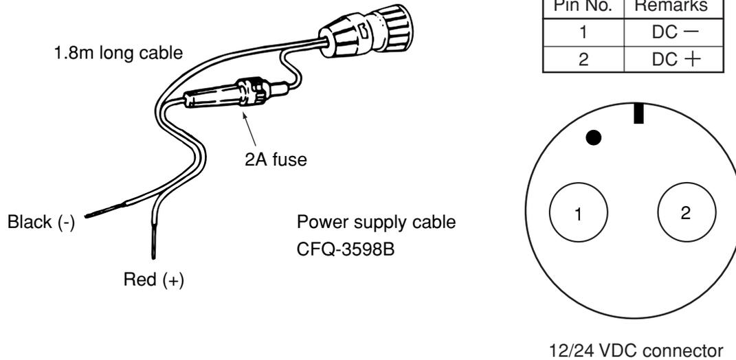
Connect the red cable to the plus terminal of the battery or power distribution panel and the black cable to the minus terminal.
