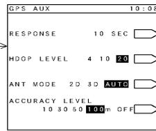
Setting the averaging for calculating the position and the speed
