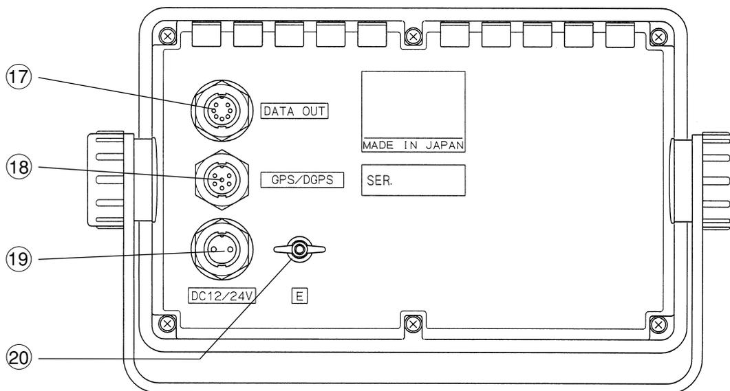
Fig. 2-2 Rear Panel of the Navigator
