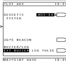
Switching the geodetic system number
