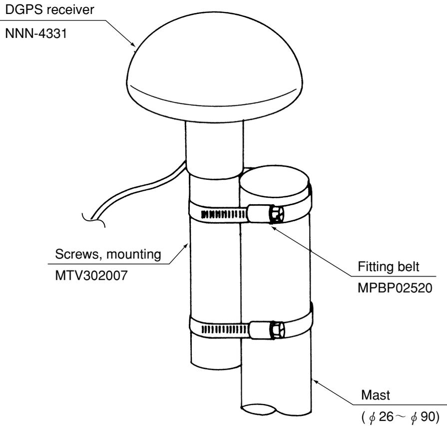
1. Loosen the fitting belt screw with a screwdriver to remove the clamp.
