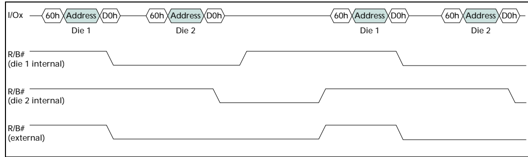
Figure 46. Interleaved BLOCK ERASE with Status Register Monitoring
