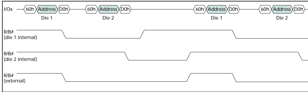
Figure 48. Interleaved BLOCK ERASE with Status Register Monitoring
