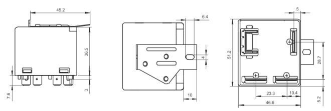
Remark: In case of no tolerance shown in outline dimension:outline dimension ≤1mm,tolerance should be 0.2mm;outline dimension>1mm and≤5mm,tolerance should be 0.3mm;outline dimension>5mm,tolerance should be 0.4mm.
