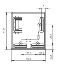
Notice: When engaging the plastic mould recess,use two flat head,self tapping screw,size 4.2mm,9.5mm long.
