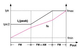
The IC operates in FM+AM mode to achieve excellent regulation and high efficiency from normal to light load conditions. When the system is near zero load, the IC operates in FM again for standby power reduction.
