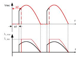
For low input condition(VIN=100~132Vac), R<sub>SET</sub> $\geq$ 66K $\Omega$  is recommend. And R<sub>SET</sub> $\leq$ 24K $\Omega$  is suitable for high input condition(VIN>176Vac).
