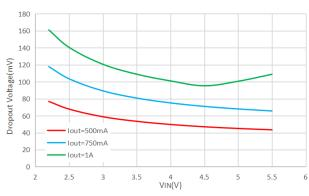
Dropout voltage vs Load current
