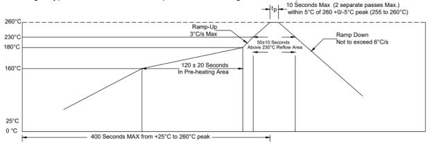
Following is typical SMD Pb-free reflow profile for soldering:
