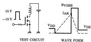
$$\begin{aligned} R_G &= 25 \ \Omega \\ V_{DD} &= 25 \ V, \ L = 165 \ \mu H \end{aligned} \qquad E_{AS} = \frac{1}{2} \cdot L \cdot I^2 \cdot \left( \frac{B_{VDSS}}{B_{VDSS} - V_{DD}} \right)$$
