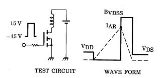
$$\begin{aligned} &RG = 25~\Omega \\ &V_{DD} = 50~V,~L = 1.74~mH \end{aligned} \qquad E_{AS} = \frac{1}{2} \cdot L \cdot I^2 \cdot \left( \frac{B_{VDSS}}{B_{VDSS} - V_{DD}} \right) \end{aligned}$$
