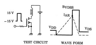
$$\begin{aligned} R_G &= 25 \ \Omega \\ V_{DD} &= 90 \ \text{V}, \ L = 7.5 \ \text{mH} \end{aligned} \qquad E_{AS} = \frac{1}{2} \cdot L \cdot I^2 \cdot \left( \frac{B_{VDSS}}{B_{VDSS} - V_{DD}} \right)$$
