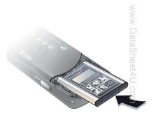
3 Insert the battery with the label side up and the connectors facing each other.
