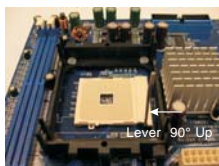
STEP 1: Lift Up The Socket Lever
