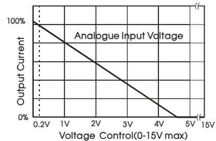
Fig. 10 Analogue input voltage and output current
