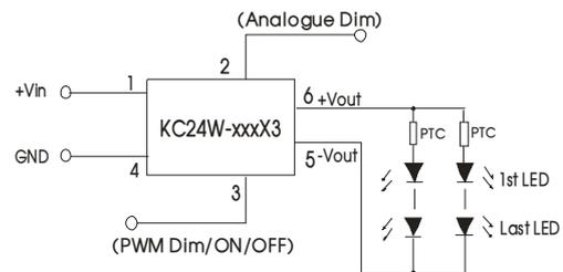
Fig. 3 Application circuits in series and parallel
