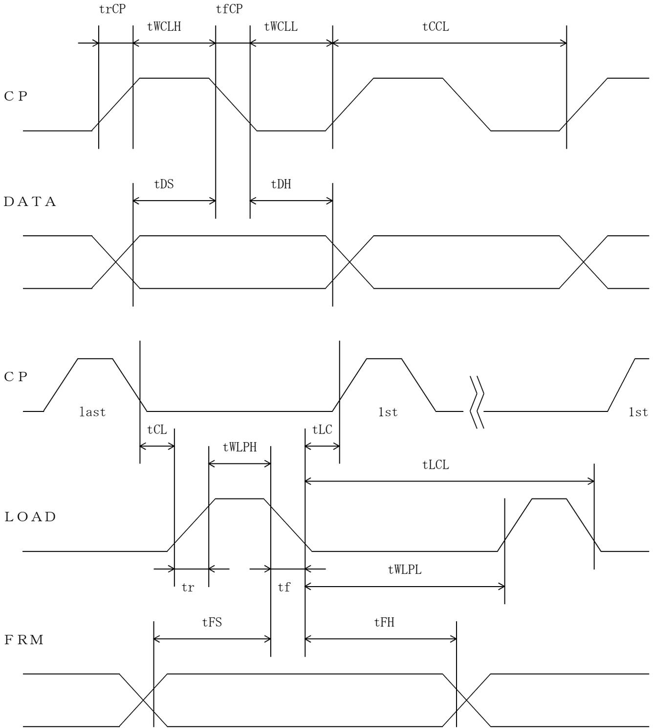
11-1. Switching characteristics (VDD=3.3V)
