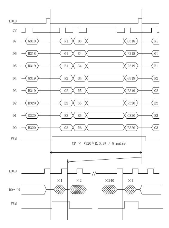
\* The cycle of load signal should be stable and continuously applied without interruption.
