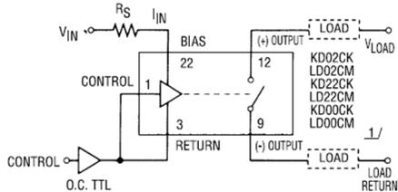
**(B) 2 Terminal Input (Open Collector TTL Drive)**
