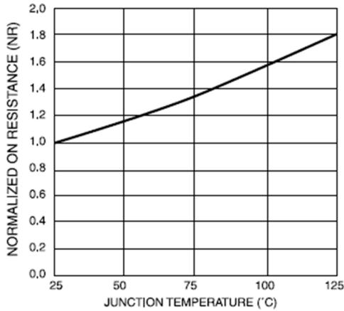
**NORMALIZED ON RESISTANCE VS JUNCTION TEMPERATURE**
