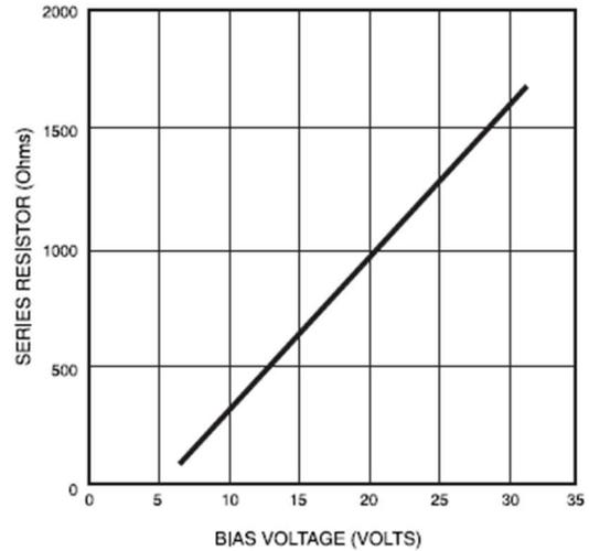
**SERIES LIMIT BIAS RESISTOR VS BIAS VOLTAGE**
