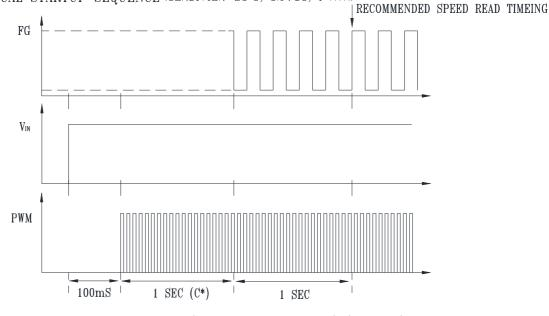
12. TYPICAL STARTUP SEQUENCE (CONDITION: 25°C, 5.0VDC, 1 ATM)
