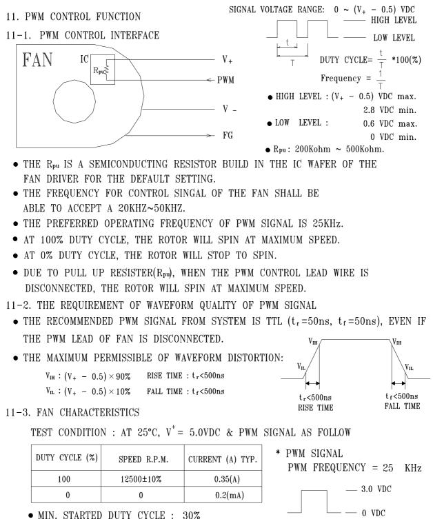
WHEN DUTY CYCLE IS SET FOR MORE THAN 30%, THE FAN WILL BE ABLE TO START FROM A DEAD STOP.
