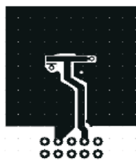
a) 87°C/W when mounted on a 1in² pad of 2 oz copper.
