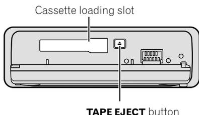
You can eject a cassette tape by pressing **TAPE EJECT**.
