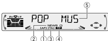
RDS (radio data system) is a system for providing information along with FM broadcasts. This inaudible information provides such features as program service name, program type, traffic announcement standby and automatic tuning intended to aid radio listeners in finding and tuning in to a desired station.
