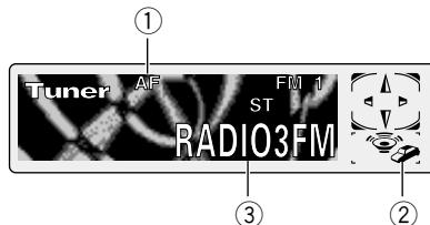
RDS (radio data system) is a system for providing information along with FM broadcasts. This inaudible information provides such features as program service name, program type, traffic announcement standby and automatic tuning, intended to aid radio listeners in finding and tuning in to a desired station.
