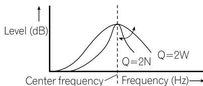
**1 Press AUDIO and hold until frequency and the Q factor (e.g., F 80 Q 1W) appears in the display.**
