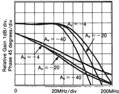
**Broadband Inverting and Non-Inverting Gain**
