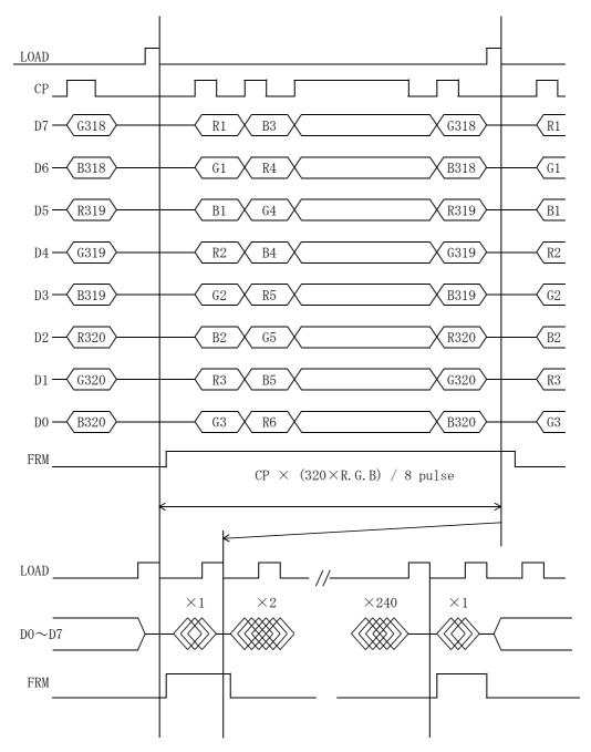
\* The cycle of load signal should be stable and continuously applied without interruption. \* The above-mentioned timing chart shows a reference to set up a LCD module, not an electrical
